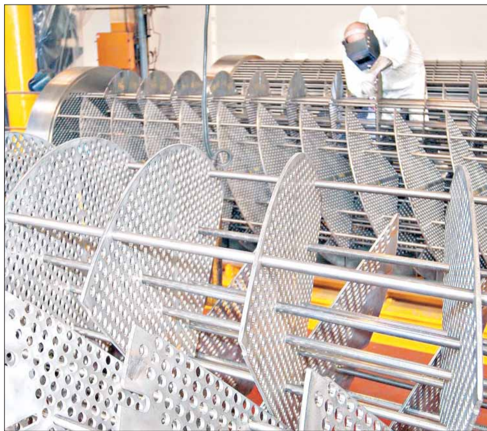
Making the new helix-shaped baffles at the Wellman works in Oldbury
